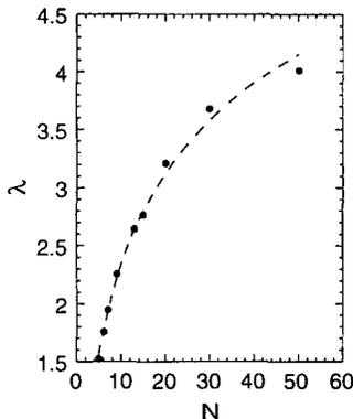
Fig. 4. Lyapunov exponent as a function of the number of scatterers in the right-bounded cavity. Dashed line corresponds to the fit proposed in Eq. (4).
