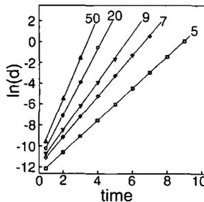
Fig. 3. Distance between parent and perturbed trajectories as a function of time (given in number of collisions). Solid lines are the fits leading to the Lyapunov exponent. Numbers on top indicate the number of scatterers in the ring cavity.
