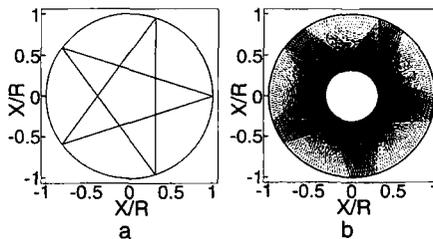
Fig. 1. Trajectories of a free particle confined to move in a smooth circular cavity. (a) Initial conditions satisfy Eq.(2); (b) Initial conditions as in (a) plus a  $10^{-2}$  perturbation in the speed.
